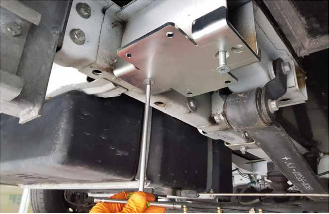
Put the adapter in the point illustrated (behind the rear axle), insert the sealing plates and fix the adapter with the M10 bolts.
