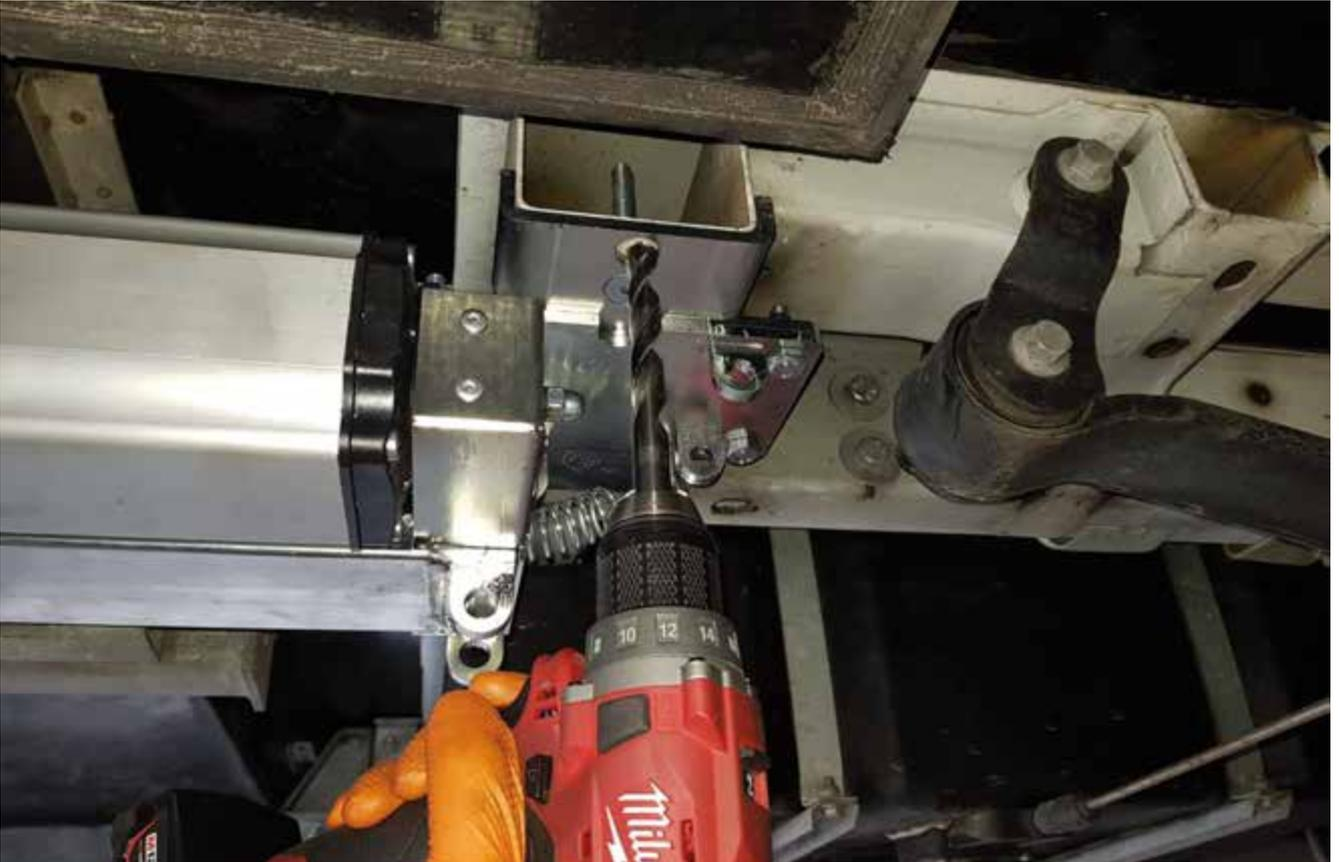
Drill a 13 mm hole through the hole in the adapter.
