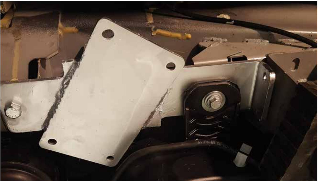
Fix the adapter with a M10 bolt and fix the support of the AdBlue tank above the adapter
