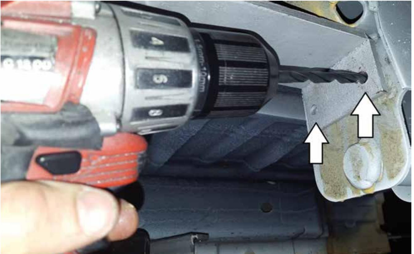
Push the adapter on the frame, then drill two 10 mm holes and fix with the bolts.
