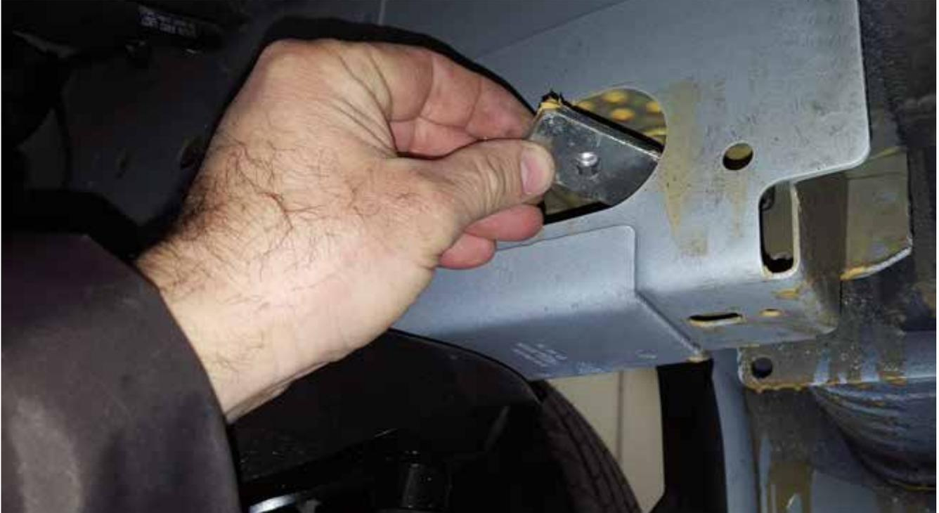
Insert the sealing plate through the hole on the frame.
